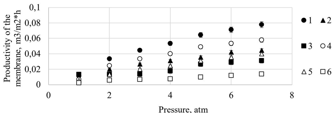
**Figure 2.** The effect of pressure on the productivity of membranes made from modified cellulose fiber, obtained with different modifiers content and at different temperature: 1 – 5%, 20 °C; 2 – 5%, 40 °C; 3 – 5%, 60 °C; 4 – 15%, 20 °C; 5 – 15%, 40 °C; 6 – 15%, 60 °C
