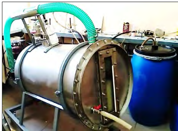
Picture 3. Biofermenter for fast and effective waste fermentation with an optimized design.
