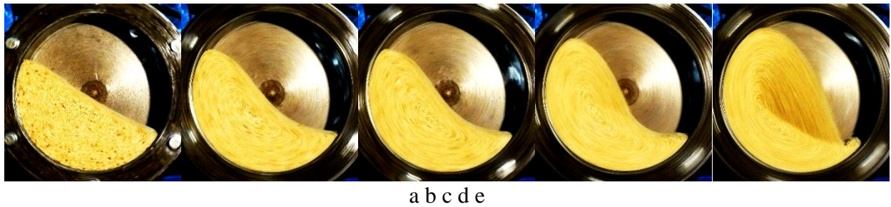
Picture 3. Visualized data of individual loading motion pictures: a – \psi_\omega=0.1 ; b – \psi_\omega=0.3 ; c – \psi_\omega=0.5 ; d – \psi_\omega=0.7 ; e – \psi_\omega=0.9
